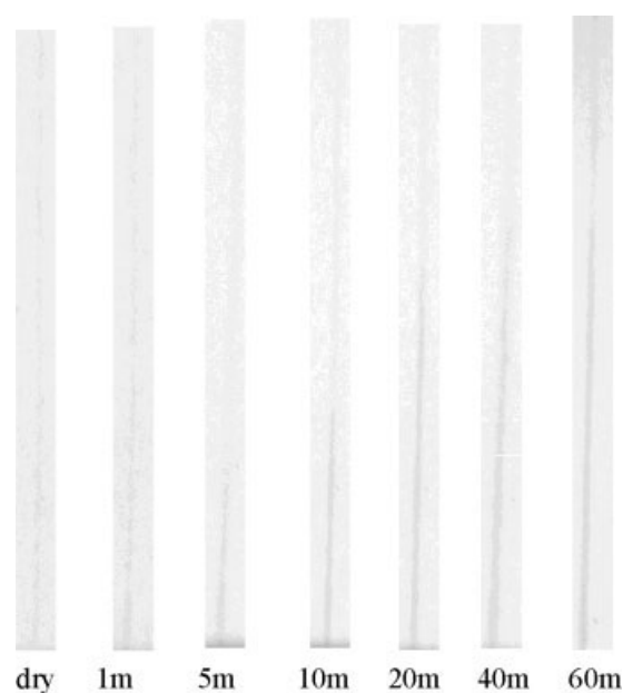
Figure 2 Radiographs of the dry and wet jute fibers for different water absorption times (1, 5, 10, 20, 40, and 60 min).
